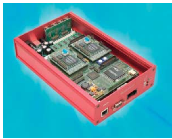
Figure 2: MoCCa Vario II evaluation board with NEC 850E/PH2 Phoenix-F
